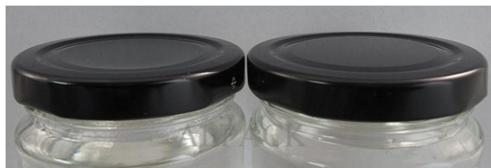
Good vacuum centre of cap pulled down.(Conave)
