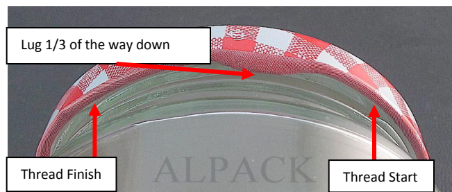
Picture shows ideal position of the cap lug on the glass thread. Approximately 1/3 of the way down the thread. Never more than half way .
