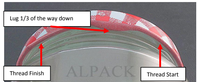
Picture shows ideal position of the cap lug on the glass thread. Approximately 1/3 of the way down the thread. Never more than half way .
