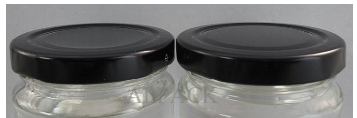
Good vacuum centre of cap pulled down.(Conave)
